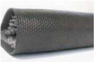
Improved rubber-backing of mats did not show any cracks after a four-week sunlight exposure test.
