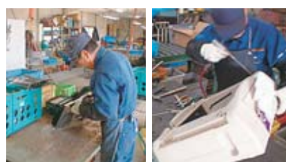
Specialized institutions disassemble and take apart each collected product by hand and one at a time.
