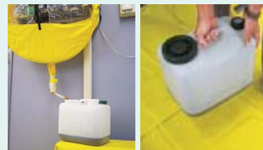
The water used in the air conditioner service is put in the tank and brought back to our shops where it is treated and discharged.
